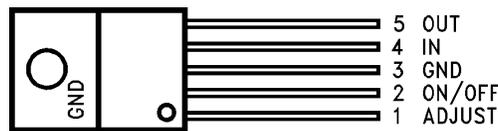
**Figure 8. TO-220 5-Lead Power Package
