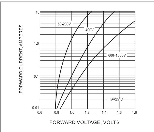
Fig.3 FORWARD CHARACTERISTICS
