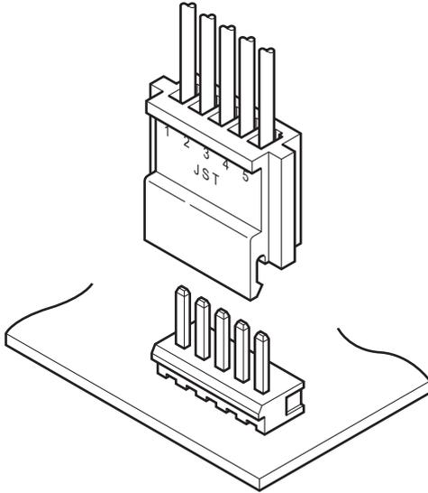
This is a 2.5 mm pitch connector for connecting PC boards and wires, and consists of a contact, housing and header. There are three types of Header: top, side and bottom entry types, which allow wires to be drawn up, down, or parallel to the PC board by combining them.
