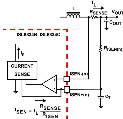
FIGURE 5. SENSE RESISTOR IN SERIES WITH INDUCTORS
