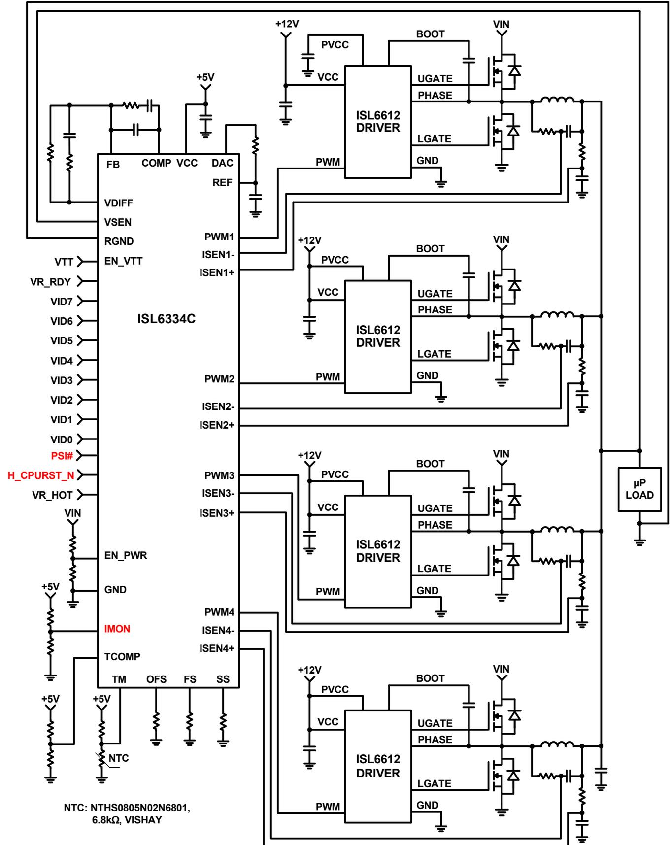
**Typical Application - CI VR with External Thermal Compensation, 2-Phase PS# (no DE and GVOT)**
