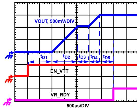
FIGURE 9. SOFT-START WAVEFORMS
