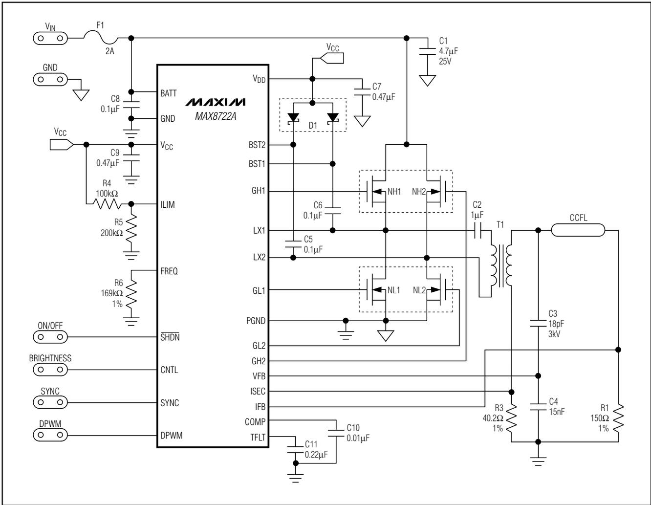
Figure 1. Typical Operating Circuit of the MAX8722A
