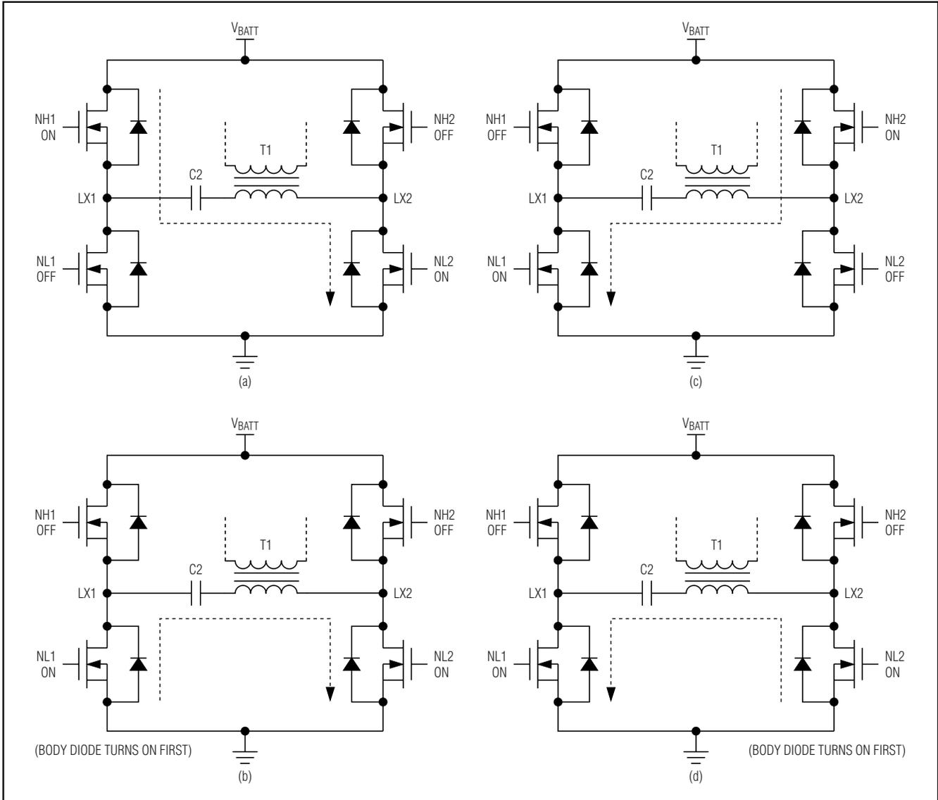
Figure 3. Resonant Operation
