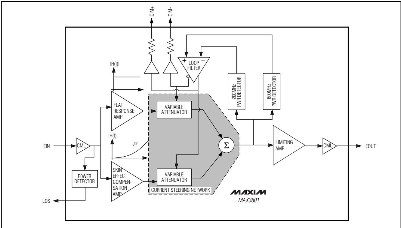
Figure 1. Functional Diagram
