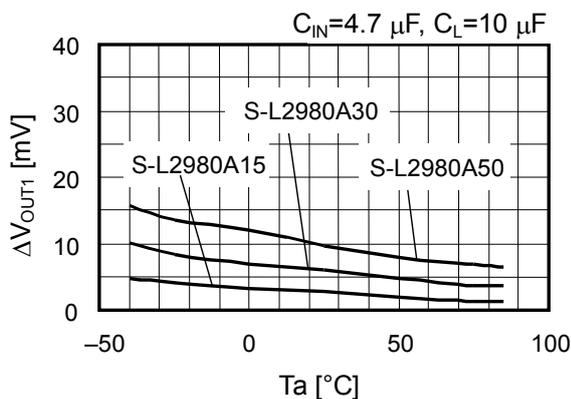
**7. Load Regulation versus Ambient Temperature**
