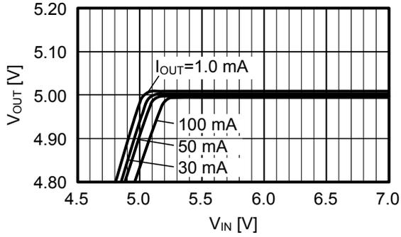
4. Dropout Voltage versus Output Voltage
