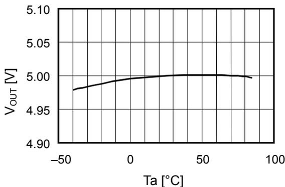
**6. Line Regulation versus Ambient Temperature**
