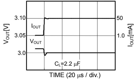
1-3. ON/OFF Switching (S-L2980A50MC, Typical data,  $T_a=25^\circ\text{C}$ )
