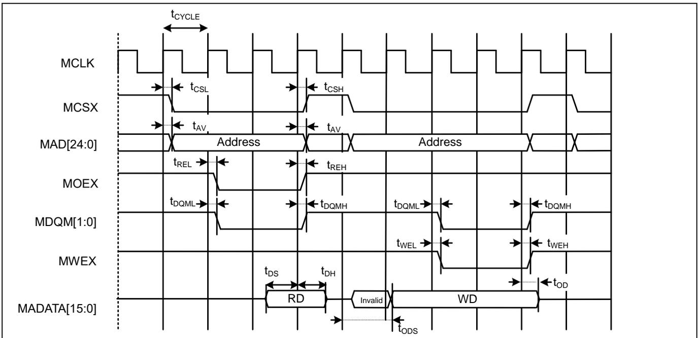
**Multiplexed Bus Access Asynchronous SRAM Mode**
