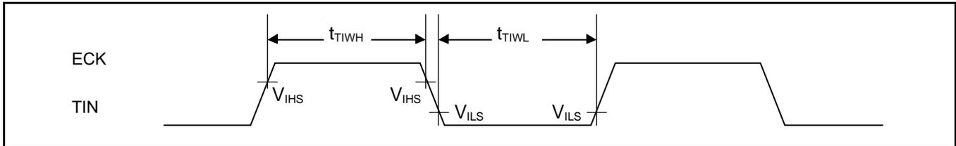
Trigger Input Timing
