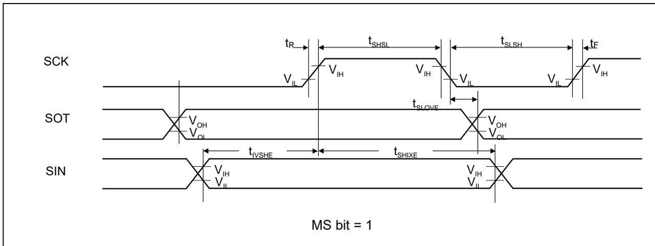
**When Using Synchronous Serial Chip Select (SCINV = 0, CSLVL=1)**
