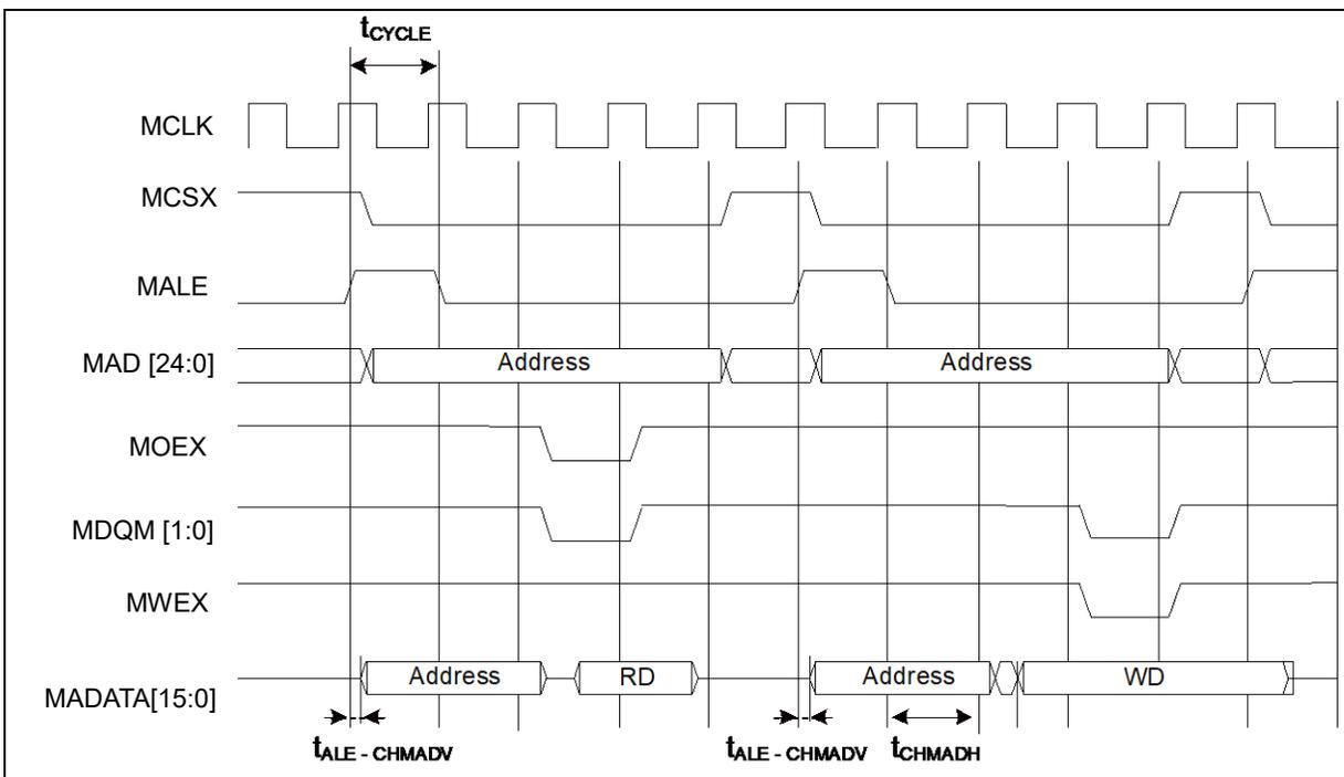
Multiplexed Bus Access Synchronous SRAM Mode
