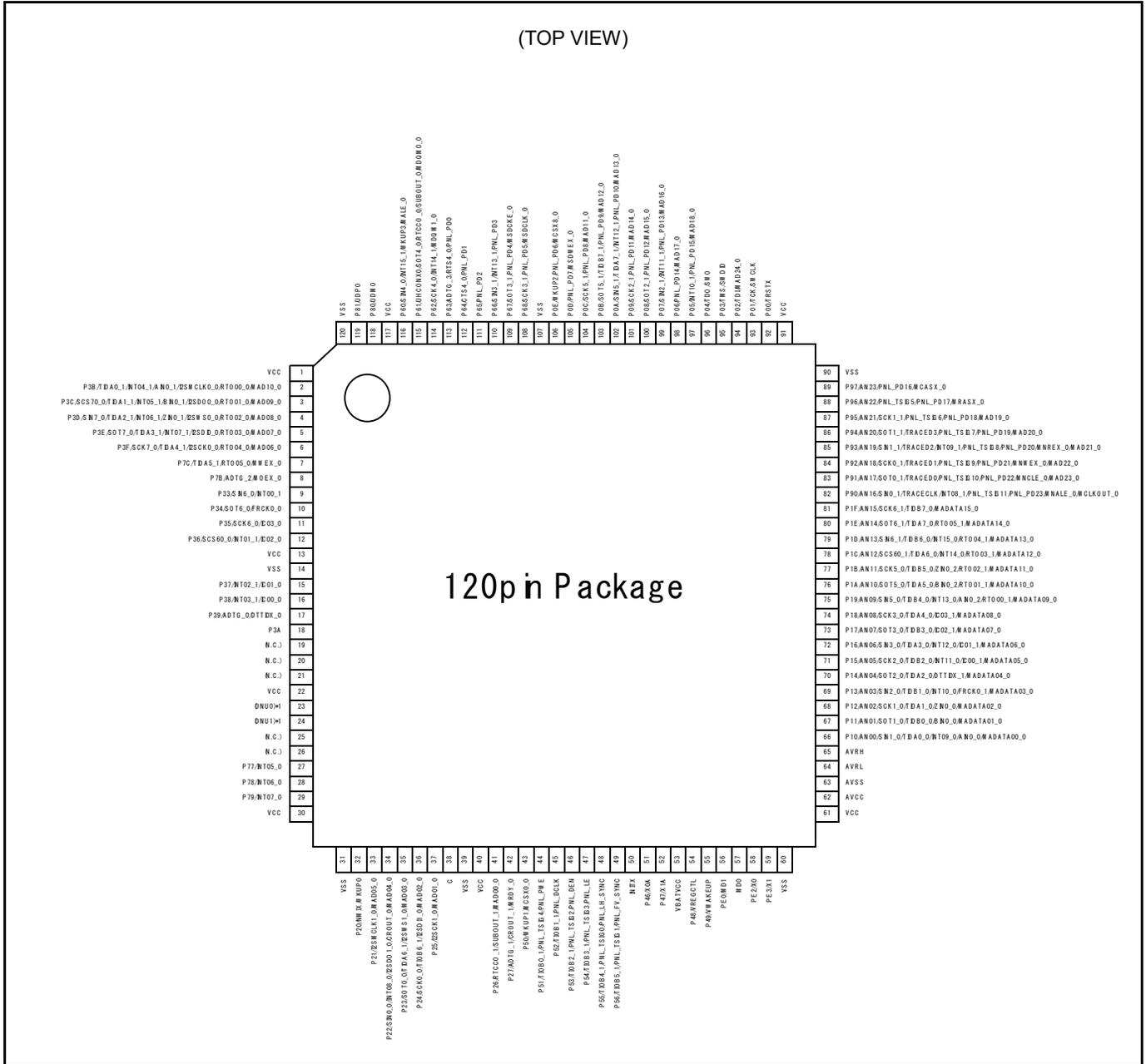
\*1: The DNU0 / 1 (23 pin / 24 pin), please pull up and short-circuit on the board.
