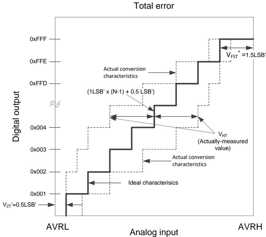
$$\text{Total error of digital output } N = \frac{V_{NT} - \{1 \text{LSB}' \times (N-1) + 0.5 \text{LSB}'\}}{1 \text{LSB}'} \quad [\text{LSB}]$$
