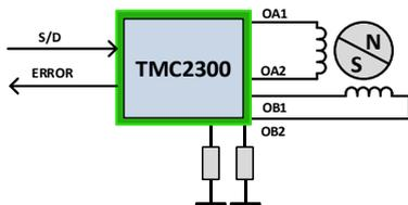
No control interface is required. The driver operates the motor based on a step & direction signal and pin-selection of the microstep resolution. In this mode, advanced stall detection and diagnostic features are not available.
