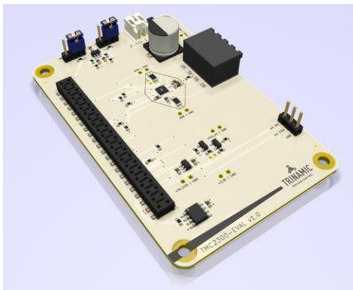
The TMC2300-EVAL is part of TRINAMICs universal evaluation board system which provides a convenient handling of the hardware as well as a user-friendly software tool for evaluation. The TMC2300 evaluation board system consists of three parts: Landungsbrücke (base board), Eselsbrücke (connector board with test points), and TMC2300-EVAL.
