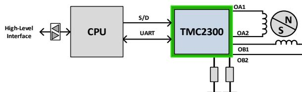
**Figure 1.3 STEP/DIR Driver with UART**
