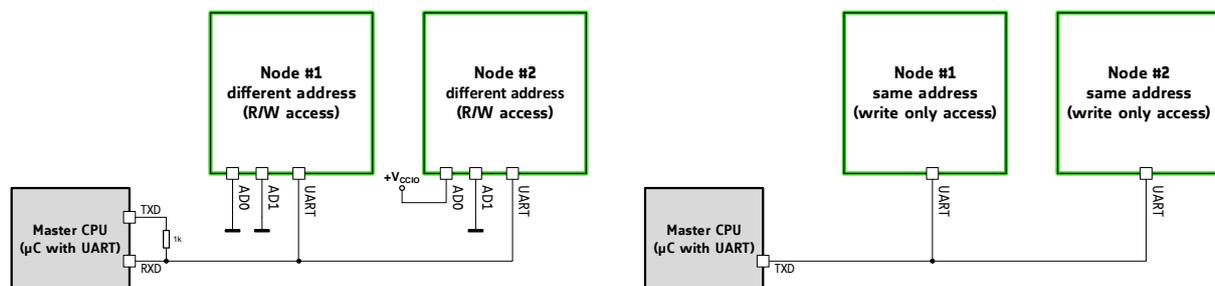
Figure 4.1 Attaching the TMC2300 to a microcontroller UART
