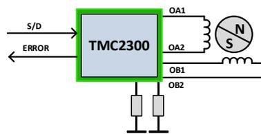
**Figure 1.2 Stand-alone driver****OPTION 2: STEP/DIR Driver with Full Diagnostics and Control**
