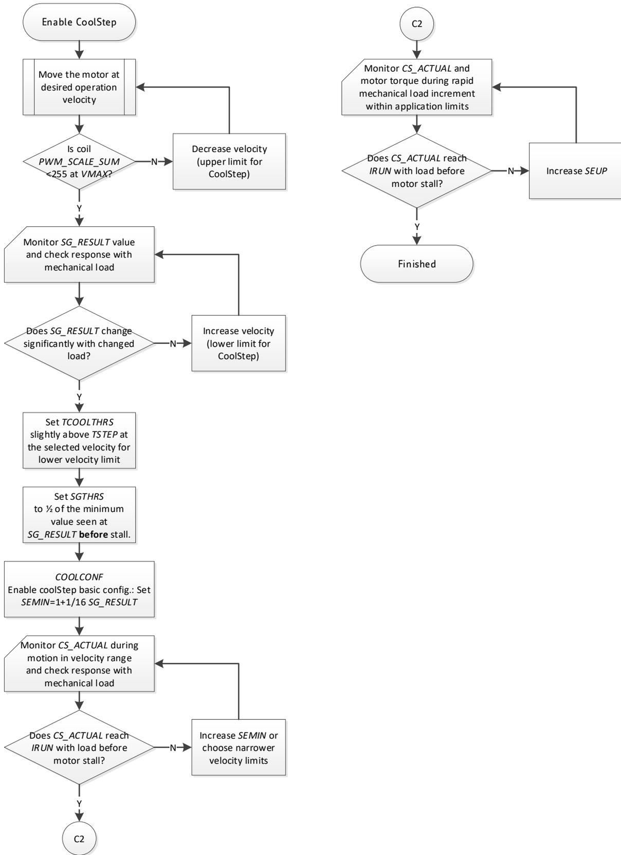
Figure 15.2 Configuration for CoolStep in StealthChop mode
