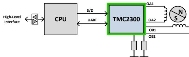
A CPU operates the driver via step and direction signals. It accesses diagnostic information and configures the TMC2300 via the UART interface. The CPU manages motion control and the TMC2300 drives the motor and smoothes and optimizes drive performance.
