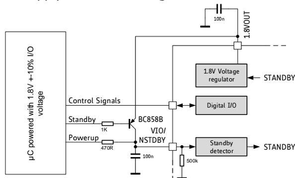
Figure 3.7 Additional Circuit for 1.8V I/O voltage
