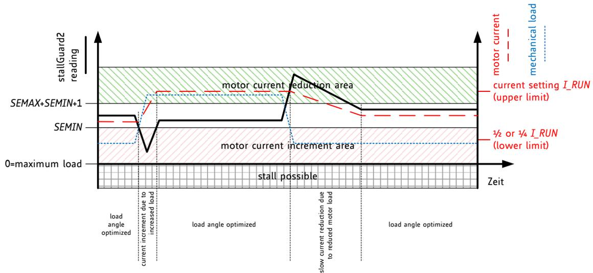
**Figure 11.1 CoolStep adapts motor current to the load**
