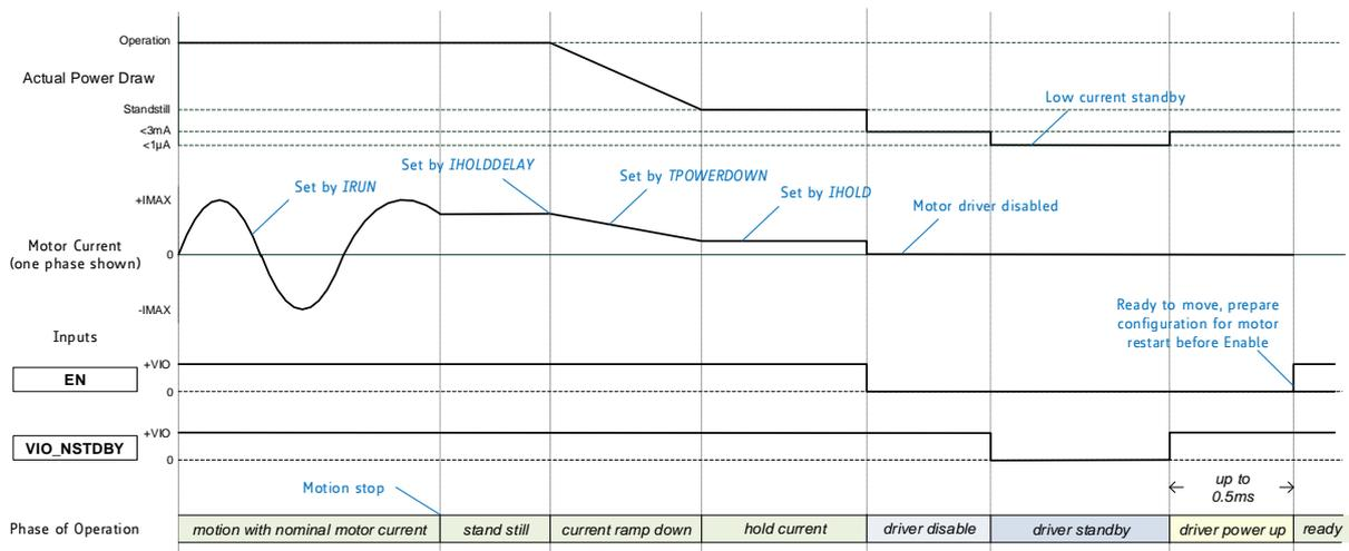
Figure 3.5 Switching to Standby and Back On
