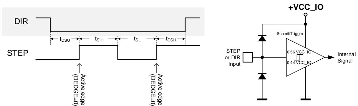
Figure 12.1 STEP and DIR timing, Input pin filter
