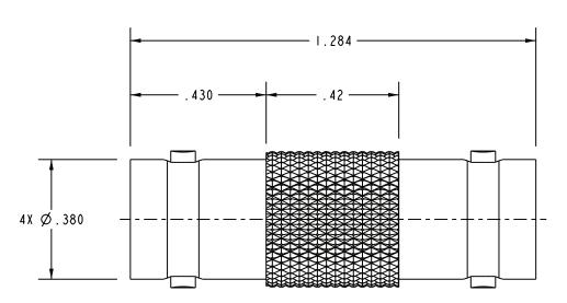
2. WITHIN SERIES FEMALE BNC FEEDTHRU ADAPTER,  $50\Omega$  AND  $75\Omega$  VERSIONS
