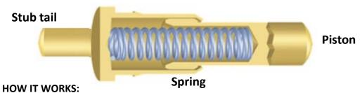
Strong, secure and featuring one piece solid body construction, there are no capped components at the bottom of this spring contact. No seams for solder to wick inside the shell.
