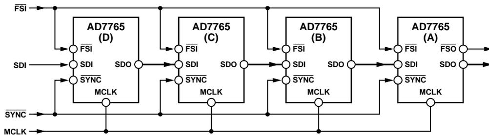
Figure 42. Writing to an AD7765 Daisy-Chain Configuration
