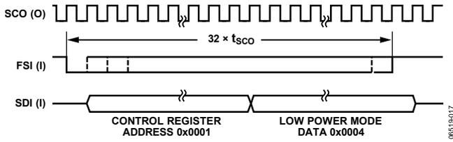
Figure 38. Write Scheme for Low Power Mode
