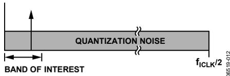
Figure 23.  $\Sigma$ - $\Delta$  ADC, Quantization Noise
