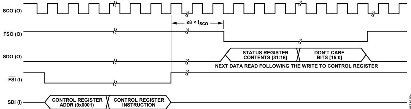
Figure 4. Status Register Read Cycle Timing Diagram
