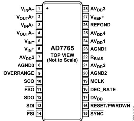
Figure 5. Pin Configuration
