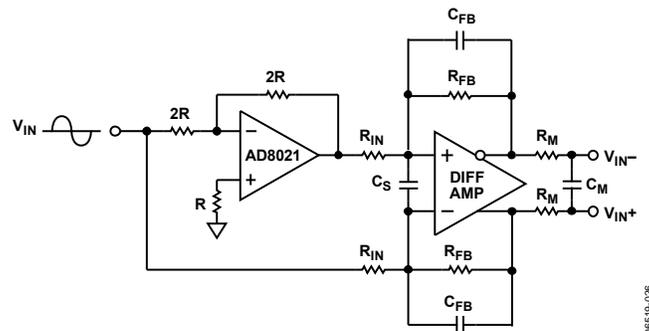
Figure 32. Single-Ended-to-Differential Conversion
