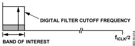
Figure 25.  $\Sigma$ - $\Delta$  ADC, Digital Filter Cutoff Frequency
