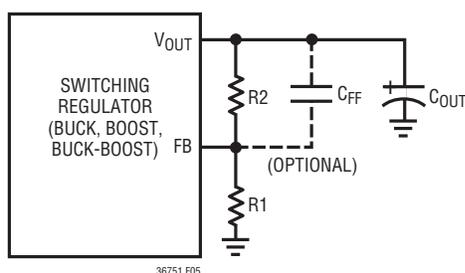
Figure 5. Feedback Components
