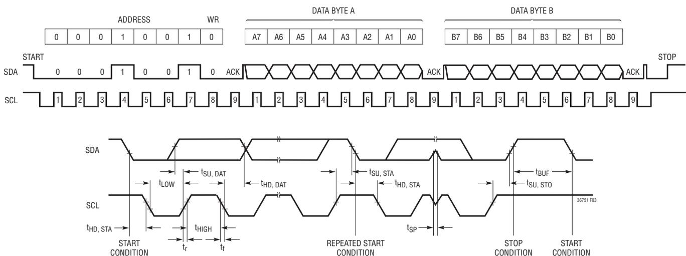
Figure 3. I<sup>2</sup>C Bus Operation
