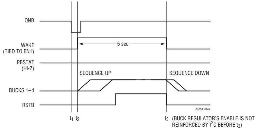
**Figure 2a. Power-Up Using WAKE (Sequenced Power-Up, Figure 7)**
