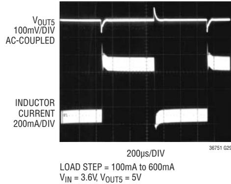
**Boost Regulator Transient Response (Burst Mode Operation)**
