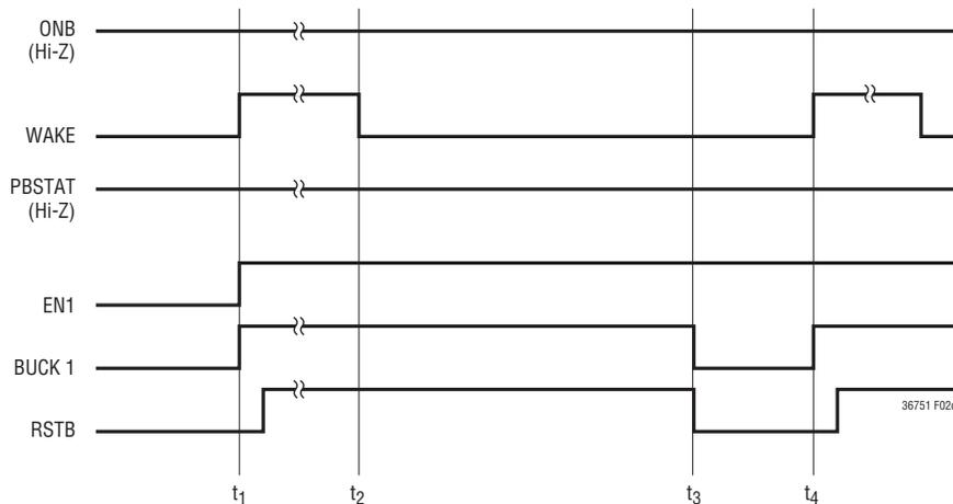
**Figure 2c. Power-Up Using an Enable Pin and Power-Down Due to I<sup>2</sup>C Generated Hard Reset**
