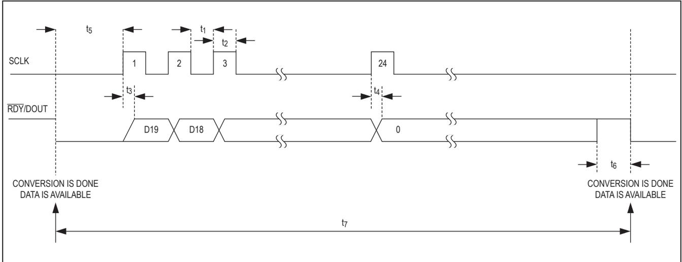
Figure 1. Timing Diagram for Data Read After Conversion
