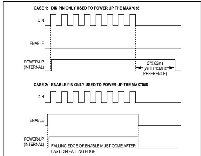
Figure 1. Power-Up Waveform with DIN/ENABLE for MAX7058
