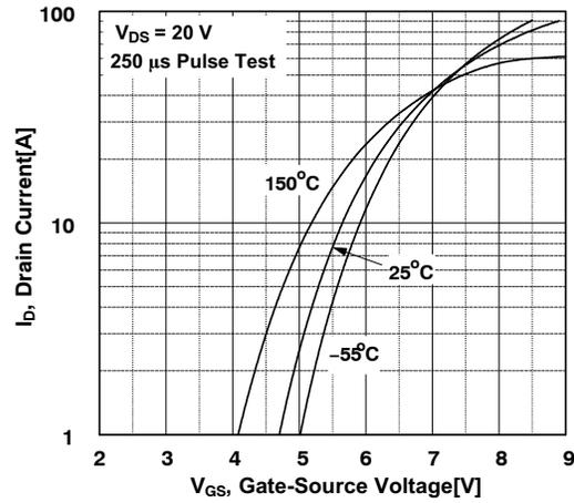
Figure 2. Transfer Characteristics
