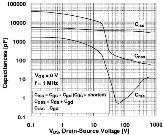
Figure 5. Capacitance Characteristics
