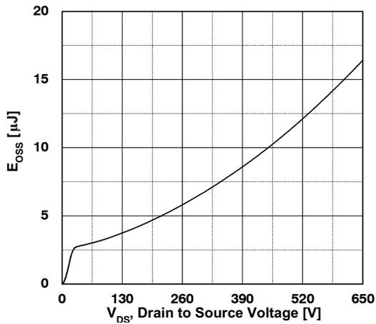
Figure 11. E<sub>oss</sub> vs. Drain-to-Source Voltage
