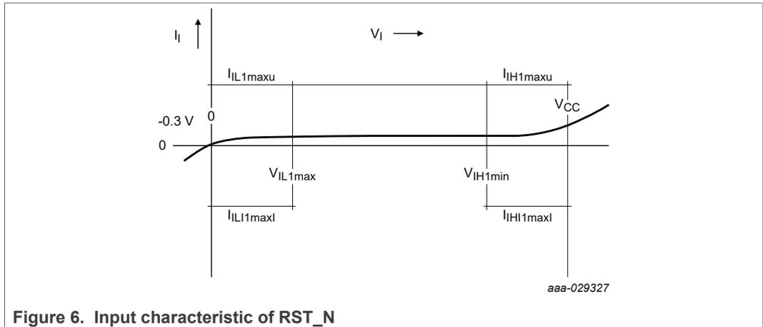
Figure 6. Input characteristic of RST\_N
