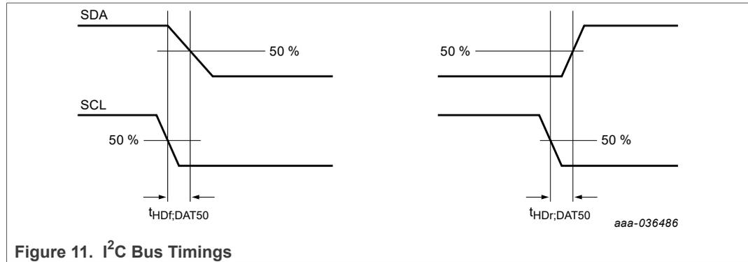
**Figure 11. I<sup>2</sup>C Bus Timings**
