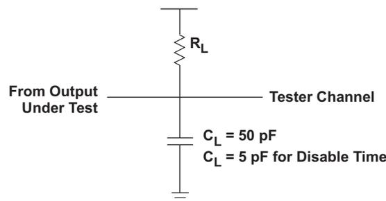
Figure 2. Test Load Circuit for AC Timing Measurements
