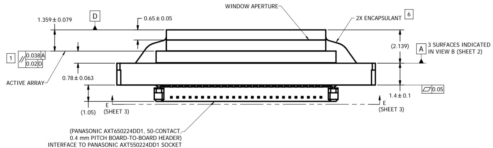
(PANASONIC AXT650224DD1, 50-CONTACT, 0.4 mm PITCH BOARD-TO-BOARD HEADER) INTERFACE TO PANASONIC AXT550224DD1 SOCKET
