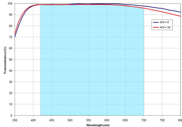
Figure 13. Corning Eagle XG Visible AR Coating Transmittance
