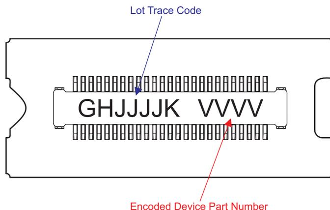
Figure 17. Device Marking
