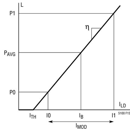
**Figure 16. Approximate LI Curve for a Laser Diode**
