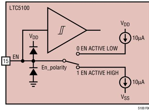
Figure 6. Equivalent Circuit for the EN Pin
