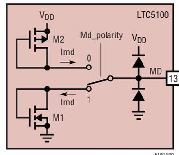
Figure 9. Equivalent Circuit for the MD Pin
