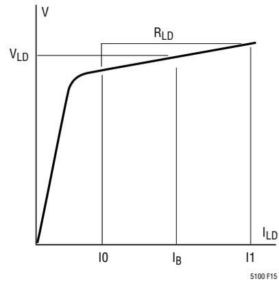
**Figure 15. Approximate VI Curve for a Laser Diode**
