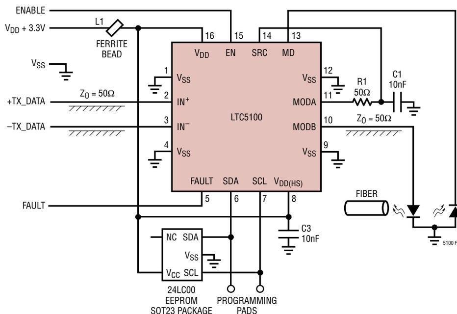
Figure 29. Schematic of a Minimum Component Count Circuit
