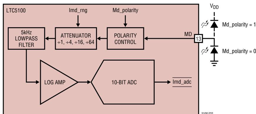
Figure 23. Detail of the Monitor Photodiode Circuit
