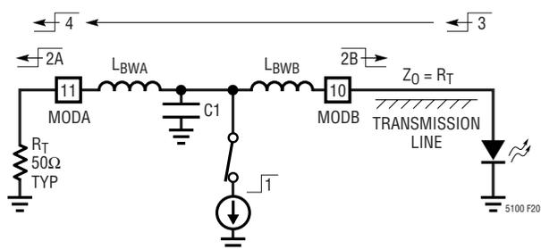
Figure 20. Wave Propagation in the Laser Interconnect
