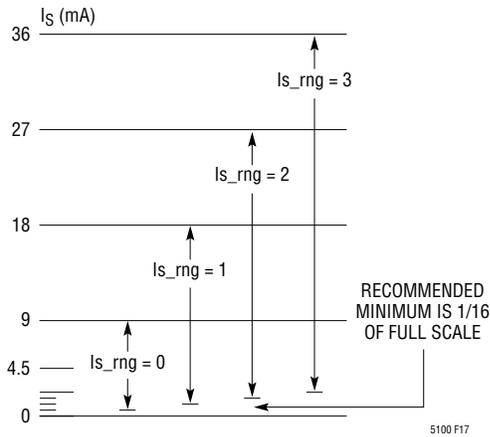
Figure 17. Ranges for the Source Current
