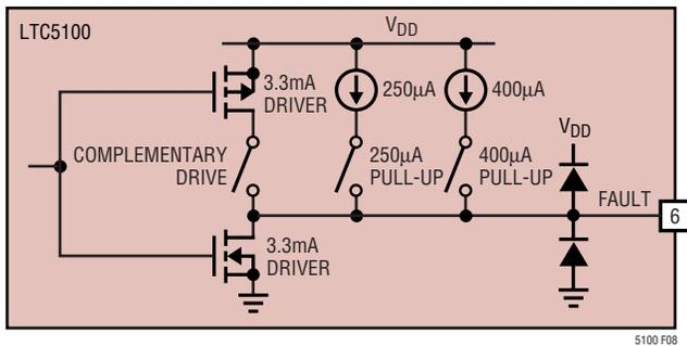
Figure 8. Equivalent Circuit for the FAULT Pin.
