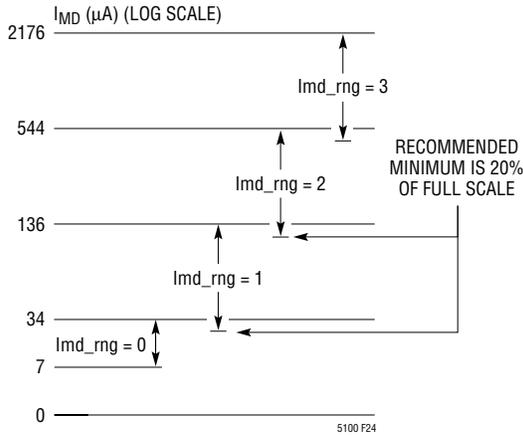
**Figure 24. Operating Ranges for the Monitor Diode Current**
