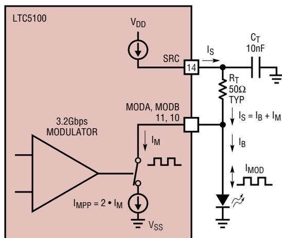
Figure 12. Simplified Laser Bias and Modulation Circuit
