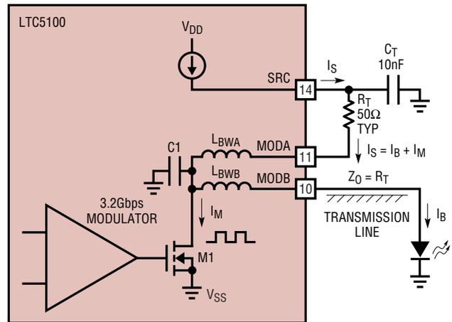
Figure 19. High Speed Details of the Modulation Output
