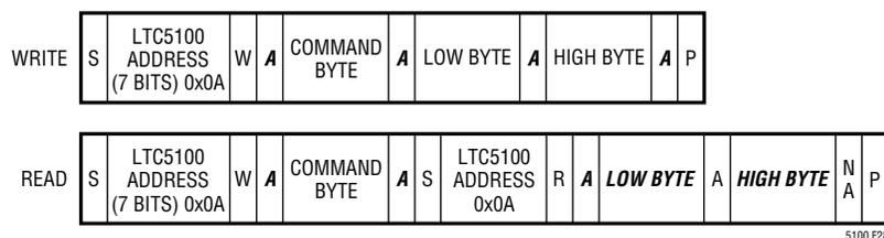
Figure 28. I<sup>2</sup>C Serial Read/Write Sequences (LTC5100 Responses are Shown in Bold Italics)
