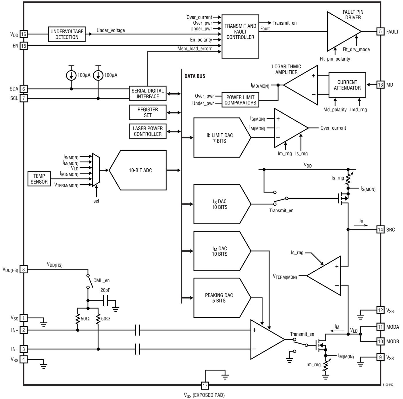
Figure 2. Block Diagram
