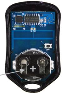
Figure 7: Battery Access
