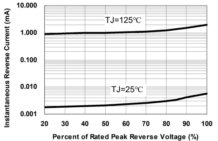
Fig.2-Typical Reverse Current
