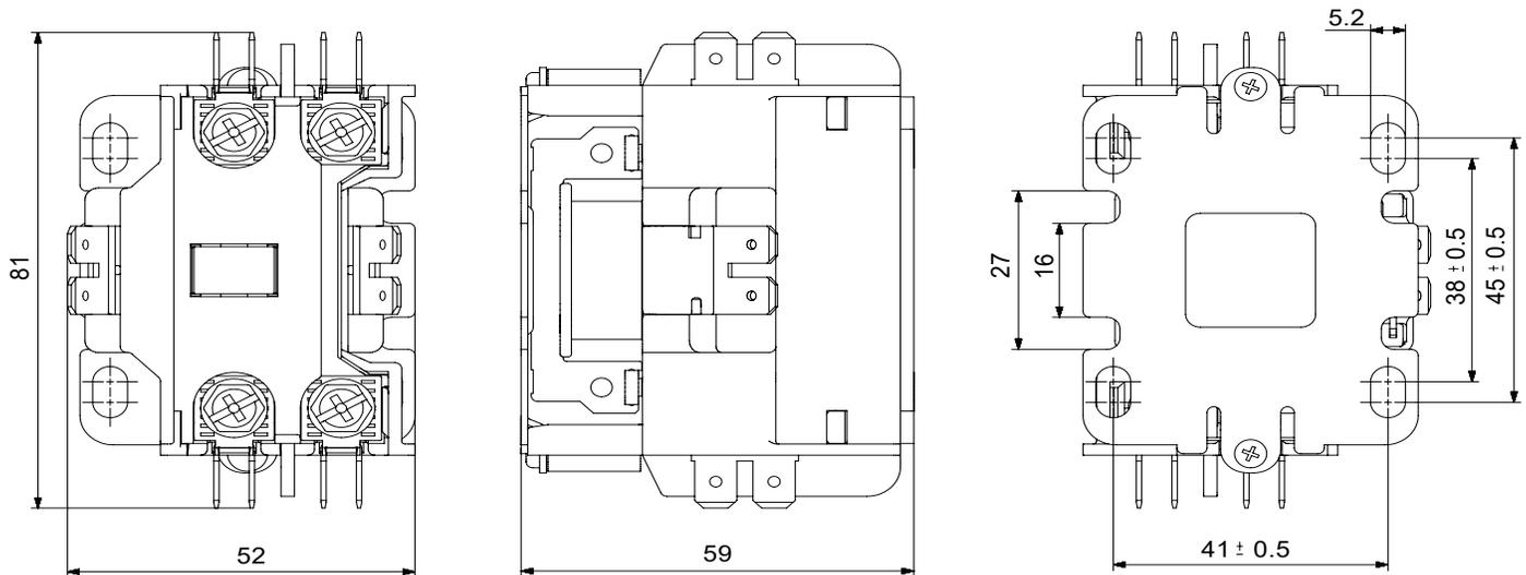
1 Pole + Shunt Contactor (Compact thermo plastic, 25-40FLA)
