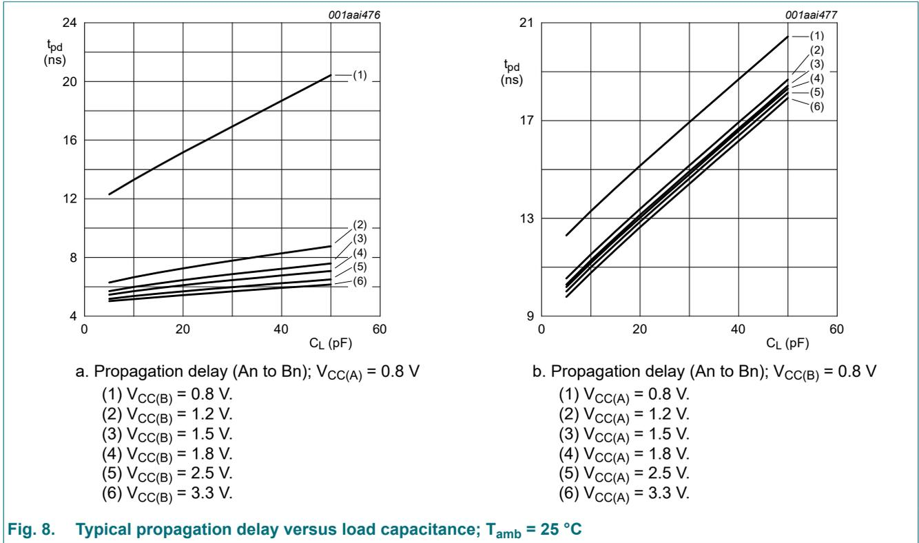
8-bit dual supply translating transceiver with configurable voltage translation; 3-state
