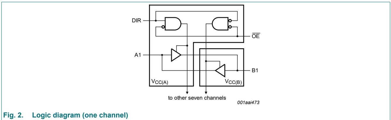
Fig. 2. Logic diagram (one channel)
