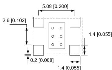
Note: Recommend using an approximately 0.01uF bypass capacitor between PIN 2 and 4.
