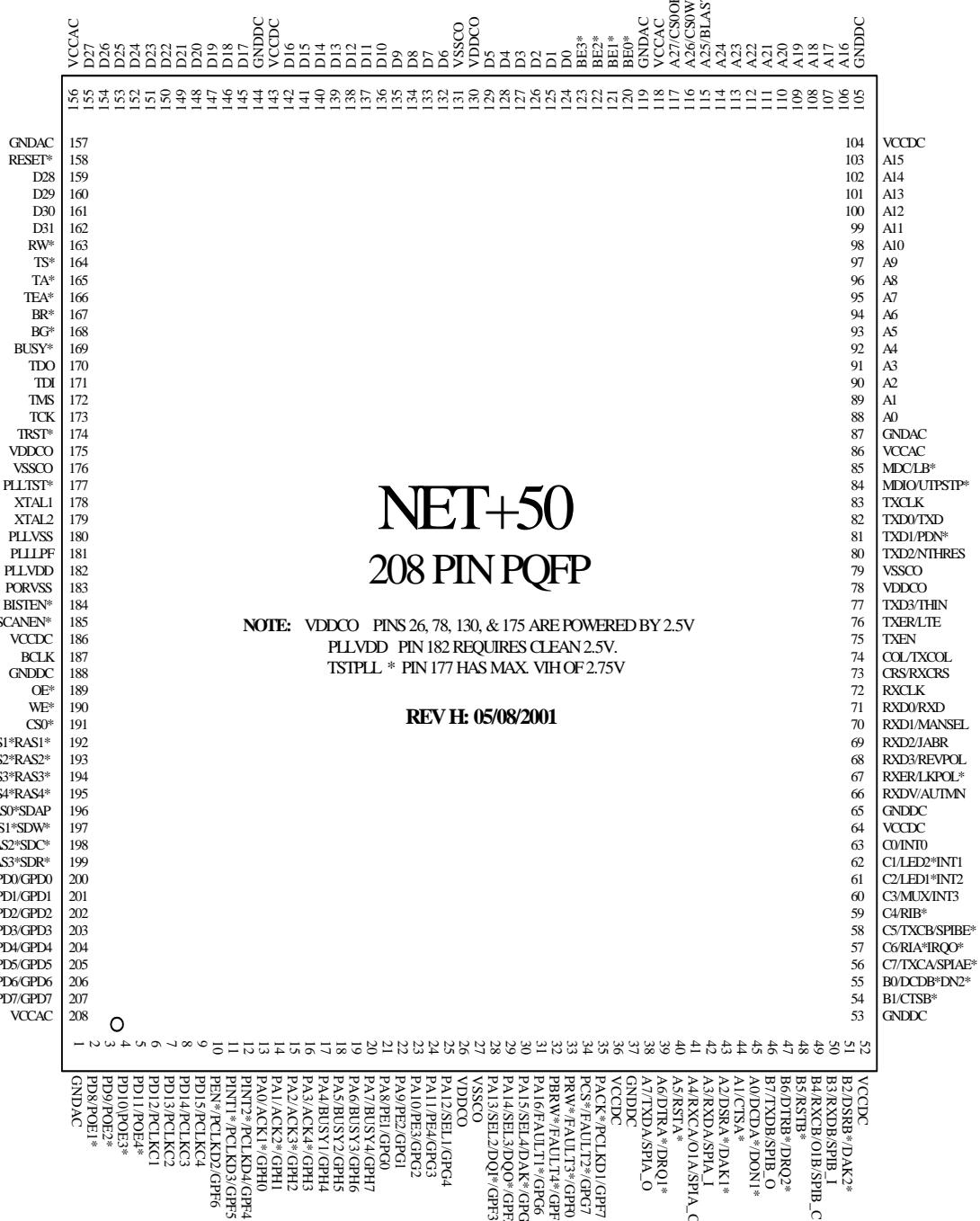
**NOTE:** VDDCO PINS 26, 78, 130, & 175 ARE POWERED BY 2.5V
