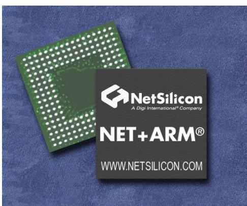
To support a variety of networking scenarios, the NET+50 includes a 10/100 BaseT Ethernet MAC with MII interface and two independent serial ports, each of which can run in UART, HDLC, or SPI mode.
