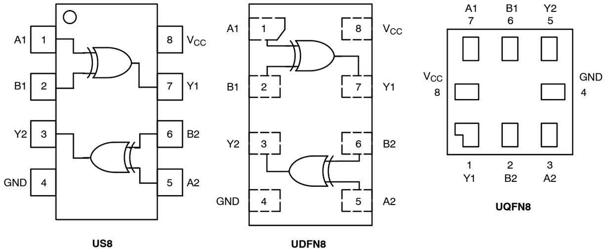
Figure 2. Pinout
