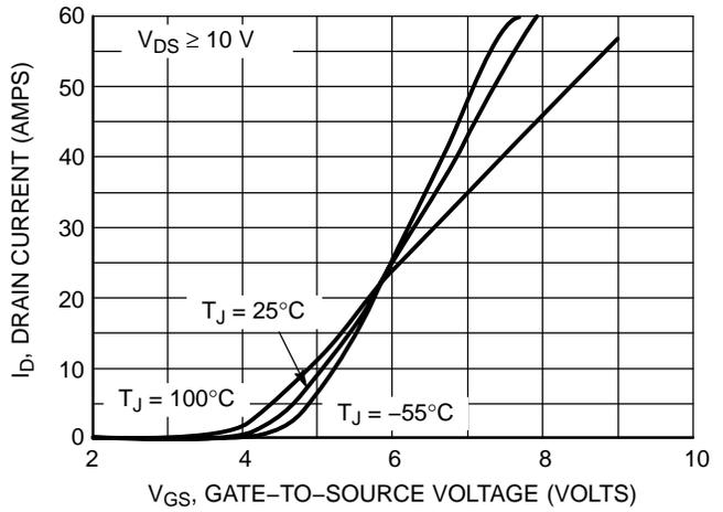
**Figure 2. Transfer Characteristics**
