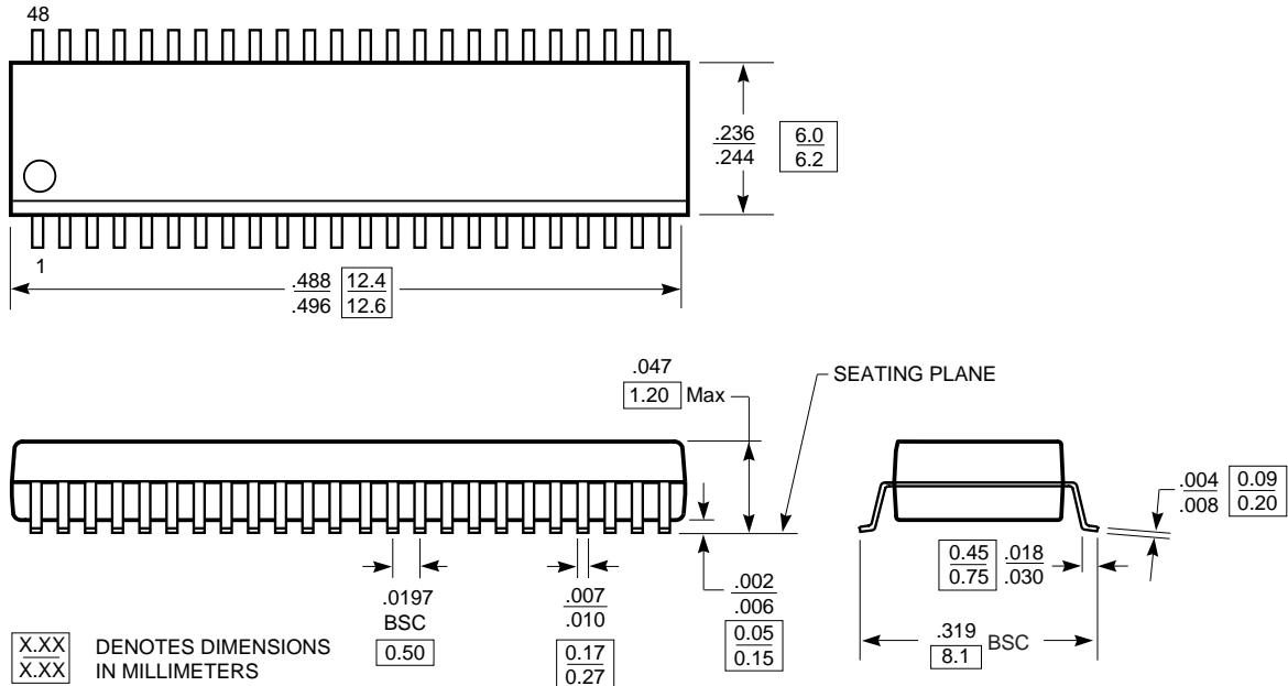
**Packaging Mechanical: 48-pin 300 mil wide plastic SSOP (V)**
