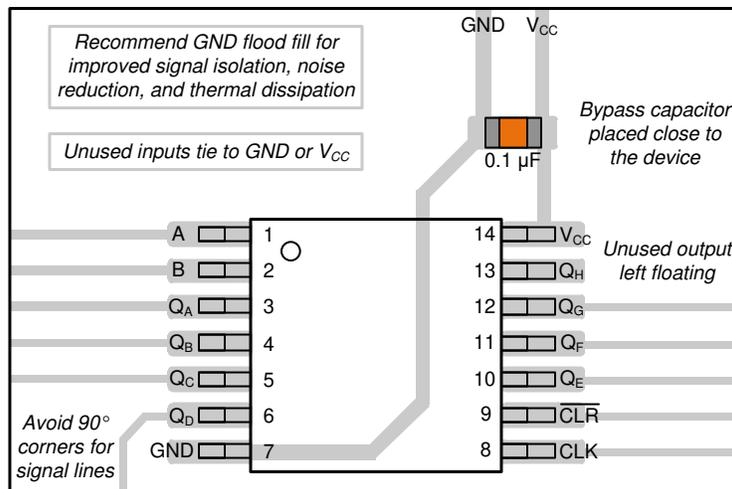
Figure 11-1. Example layout for the SN74HCS264.
