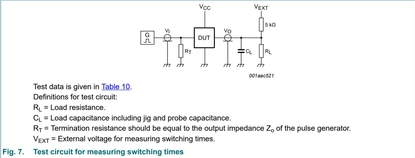
**Fig. 7. Test circuit for measuring switching times**
