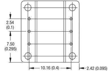
Pin Connections 76250EN (Top View)
