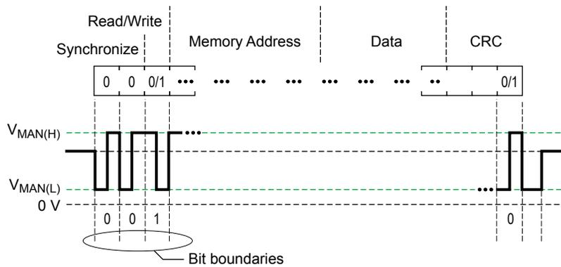
Figure 10: General Format for Serial Interface Commands
