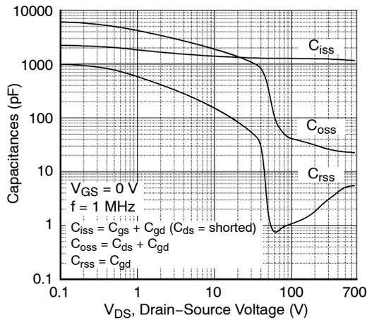
Figure 5. Capacitance Characteristics
