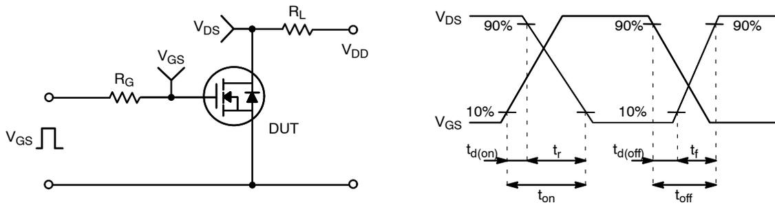
Figure 14. Resistive Switching Test Circuit & Waveforms
