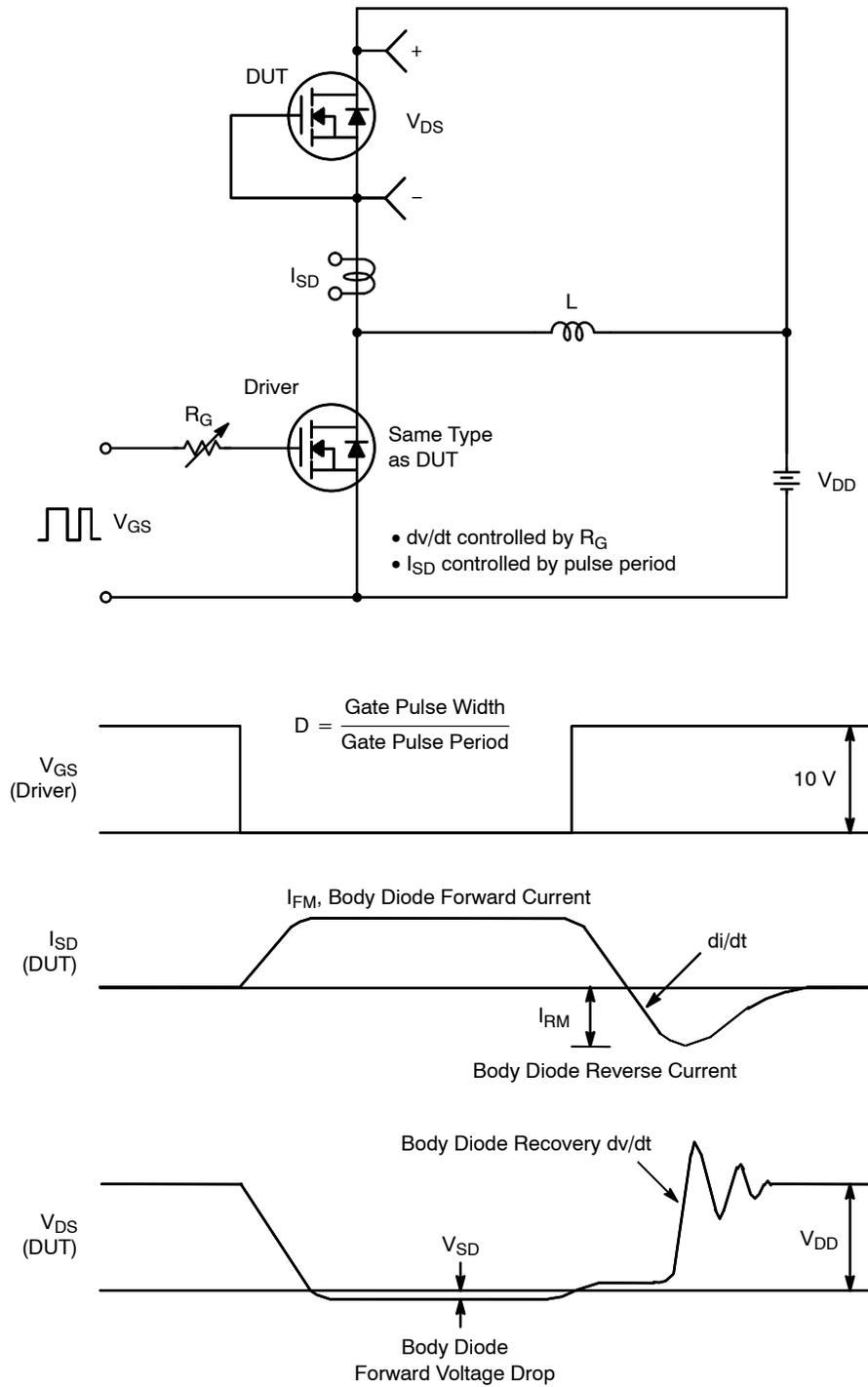
**Figure 16. Peak Recovery  $dv/dt$  Test Circuit & Waveforms**
