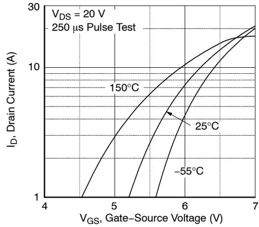
Figure 2. Transfer Characteristics
