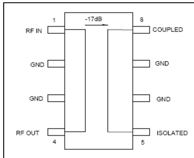
1. Pins 2, 3, 6 and 7 must be RF and DC grounded.
