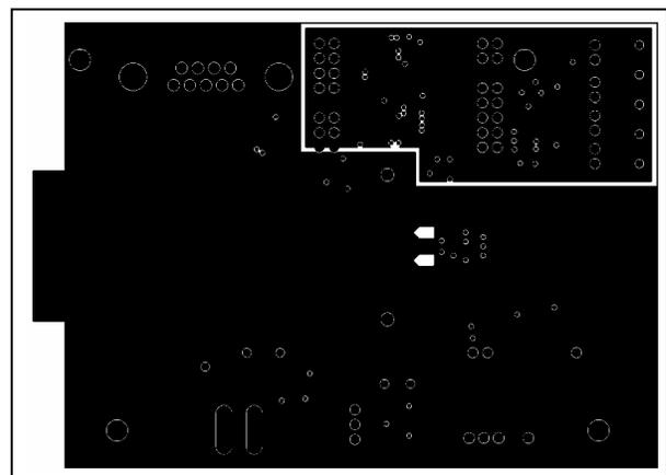
Figure 7. PC Board Layout – Ground Plane
