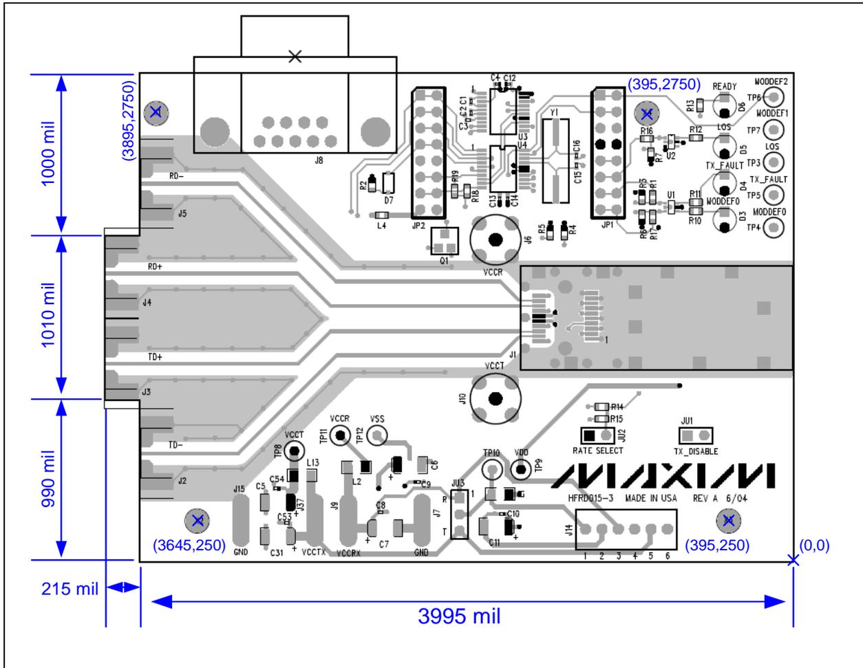
Figure 5. Host Board Dimensions / Layout
