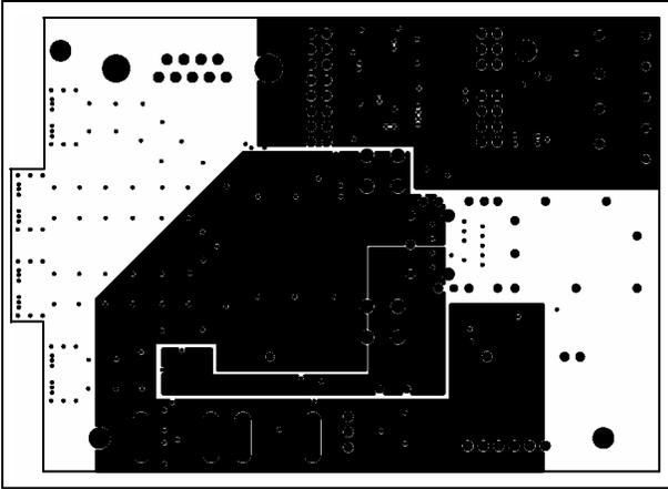
Figure 8. PC Board Layout – Power Plane
