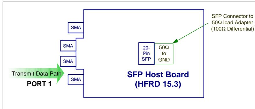
Figure 2. S11 Measurement Setup
