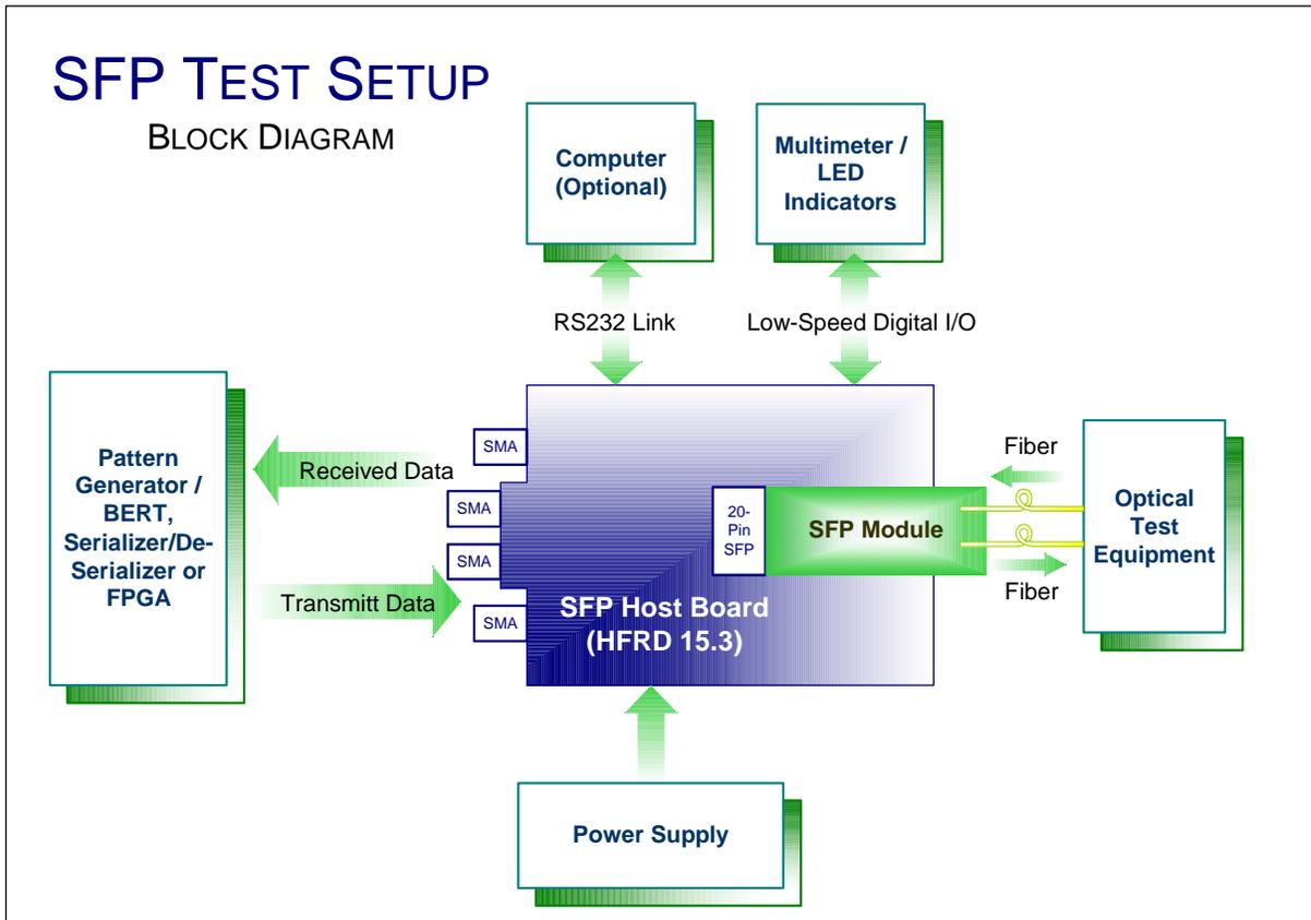
Figure 1. SFP Test Setup (Block Diagram)
