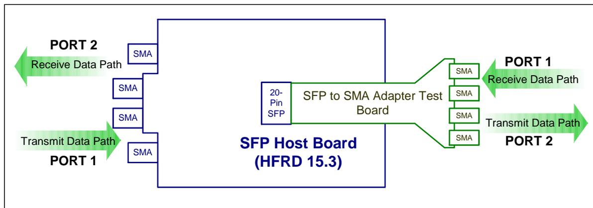
Figure 3. S21 Measurement Setup
