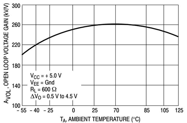
Figure 7. Open Loop Voltage Gain versus Temperature
