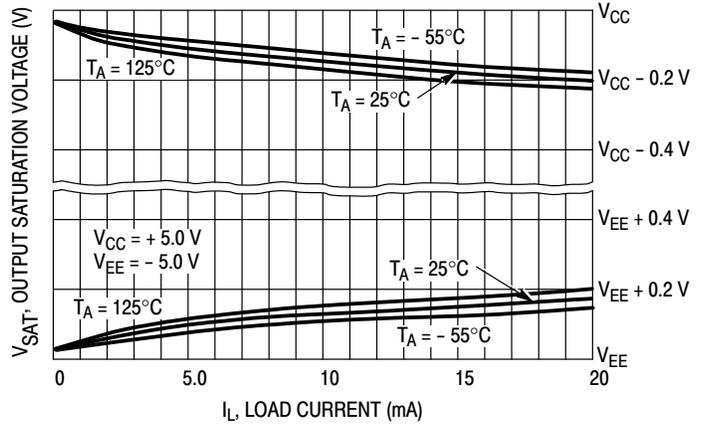
Figure 9. Output Saturation Voltage versus Load Current
