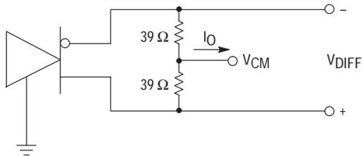
**Figure 7. AUI Differential Output Short Circuit Current**
