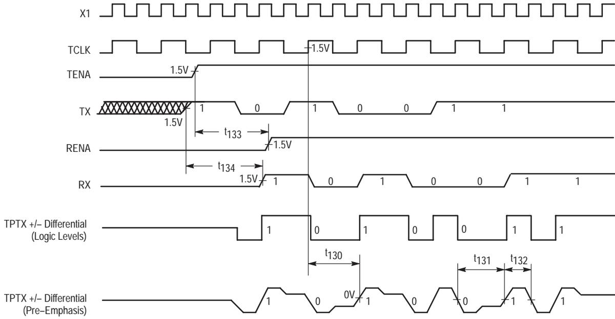
**Figure 25. TPTX Transmit Timing (End of Frame) Switching**
