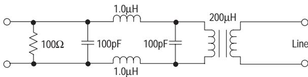
Figure 31. TPRX Input Switching
