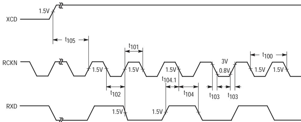
Figure 17. Receive Timing (Fujitsu End of Frame)
